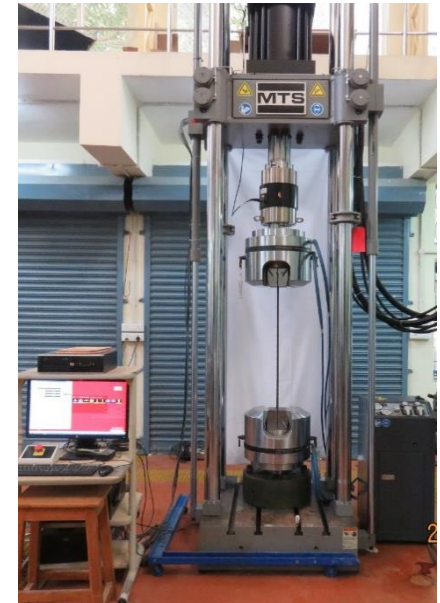
MTS servo-hydraulic tension machine
