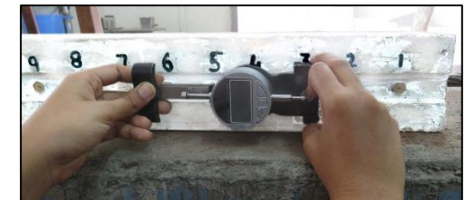
Measurements using DEMEC
