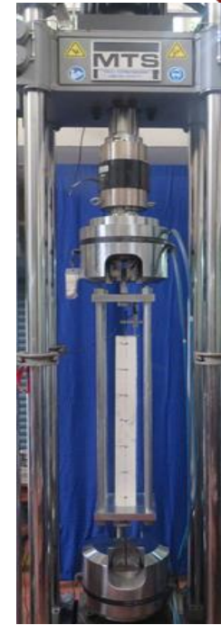
MTS servo-hydraulic tension machine
